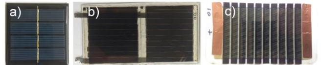
Fig. 8. PV module types: a) Silicon, b) CdTe (cadmium telluride), c) OPV.
