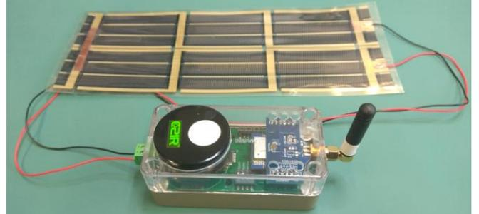
Fig. 7. Wireless sensor node with LoRaWAN RF module powered by an organic solar module.
