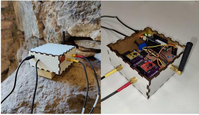
Fig. 3 Components inside the electrical enclosure (10x10x4.6 cm)
