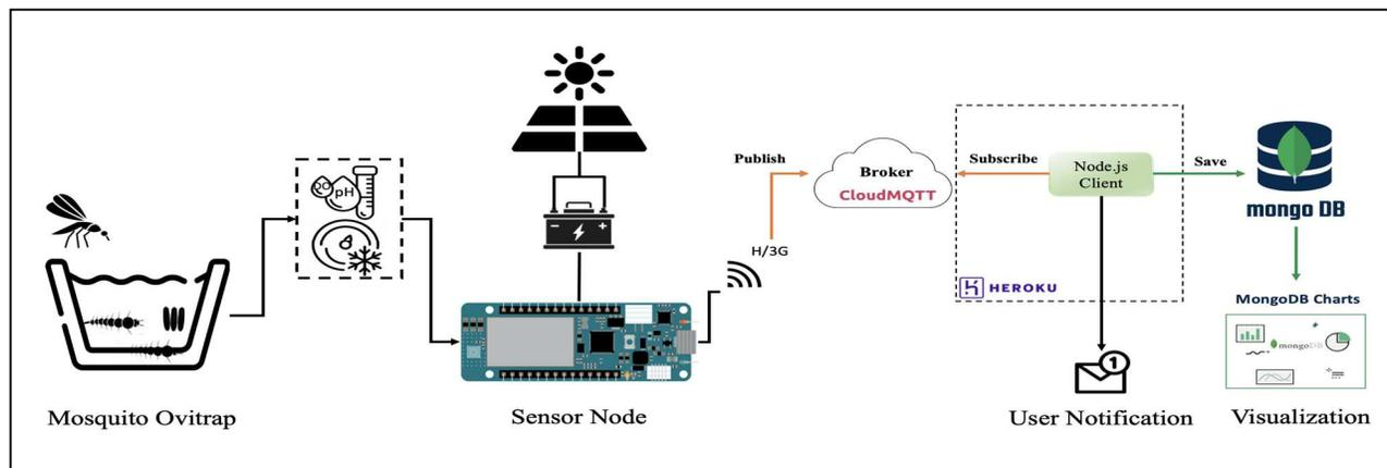
Fig. 1 MOISS architecture. It depicts how data is continuously captured from ovitraps in the field and automatically uploaded to the cloud server.
