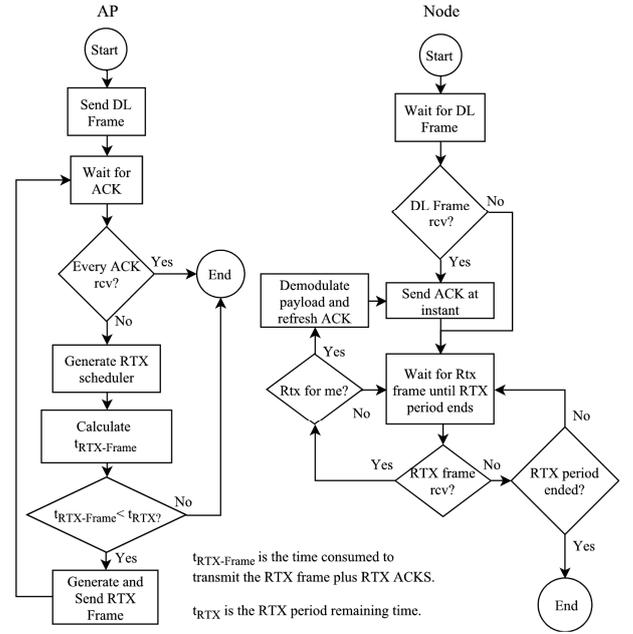
Fig. 3. DL retransmission flowchart.
