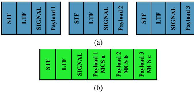
Fig. 5. Comparison between 802.11g (a) and SHARP DL PHY.
