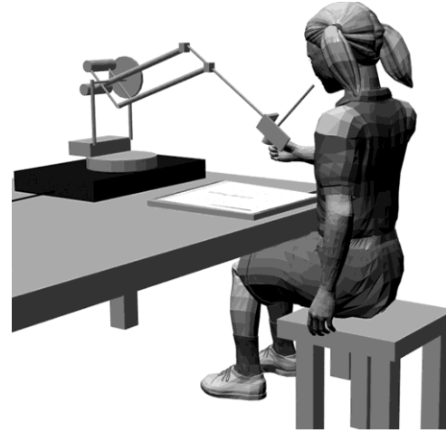
Fig. 1. Global and schematic view of the Telemaque working station. Children were seated in front of a table upon which the letters generated by the visuo-haptic interface were displayed on a horizontal computer screen. Children had to hold a pen attached to force-feedback arm controlled by the Telemaque software.
