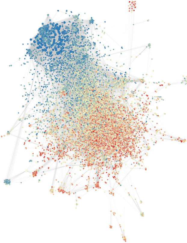
Figure 2. Absolute error in estimated distances in the CA-HEPPH dataset from low (blue) to red (high) with 100 landmarks using degree centrality .
