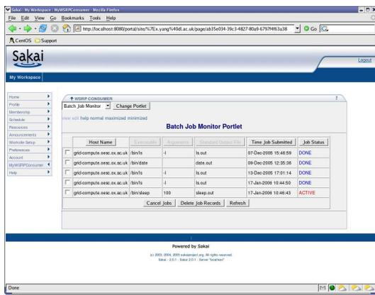
**Figure 3. Monitoring remote job status in a remote JSR 168 portlet inside Sakai via WSRP.**
