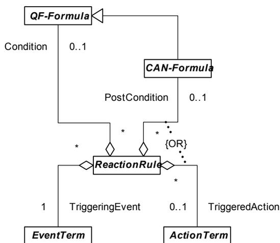
Figure 6: The general format of reaction rules.
