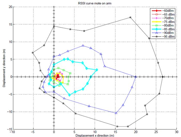
Fig. 1. RSSI contour for arm worn monitoring device
