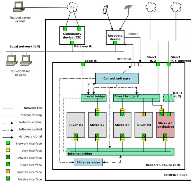
Fig. 1. The architecture of a Community-Lab node.
