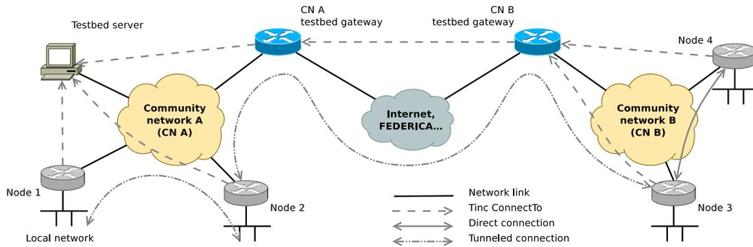
Fig. 2. The IPv6 overlay spanning two community networks.
