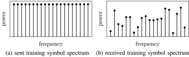
Figure 1: Channel frequency response estimation through training symbols.
