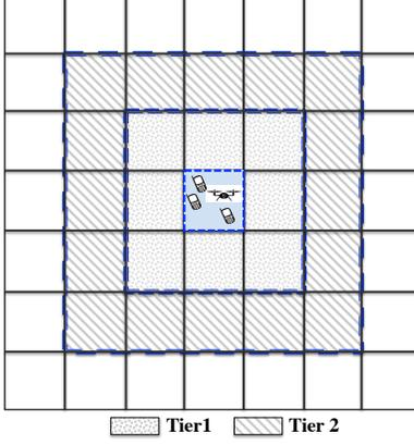
Figure 2: Multi-drone multi-user system containing 49 square cells
