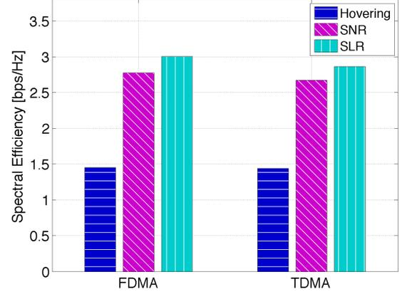
Figure 3: Spectral efficiency for both hovering drone BSs and dynamic repositioning drone BSs at low altitude  $h = 10\text{m}$
