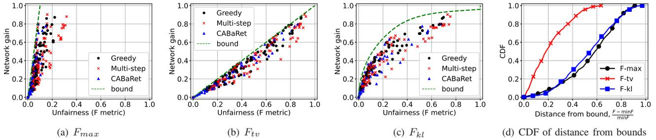
Fig. 2: (a),(b),(c): Network gain  $G$  ( $y$ -axis) vs. fairness metric  $F$  ( $x$ -axis) in all scenarios of Table II with  $C = 10$ , and under the *Greedy* (circles), *Multi-step* (crosses), *CABAret* (triangles) NF-RS. The bounds are denoted with dashed lines. (d): CDF of the relative distance  $\frac{F - \min F}{\min F}$  of the operating points  $(F, G)$  of the NF-RS algorithms from the corresponding bounds ( $\min F, G$ ).
