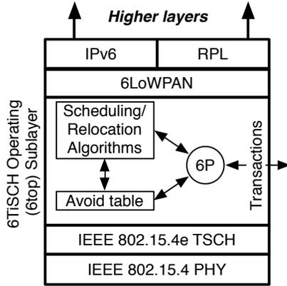
Fig. 1. TSCH integration with the IETF IoT stack
