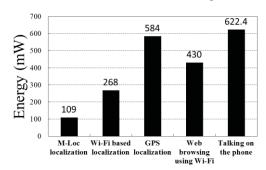
Fig. 15. The power consumption of M-Loc
