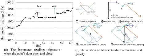
Fig. 3. The sensor readings of the smartphone on the train
