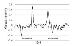
(c) The combination of the accelerometer readings variation in three axis
