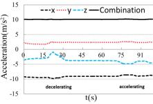
(c) The acceleration readings when the phone is randomly placed
