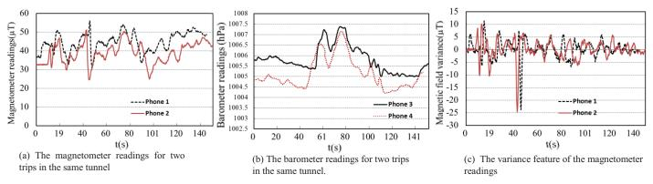
Fig. 10. The reading patterns of magnetometer and barometer in tunnels
