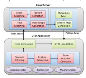
Fig. 16. Software architecture of M-Loc
