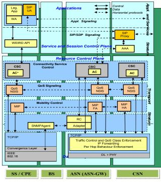
Figure 3. High Level WEIRD architecture
