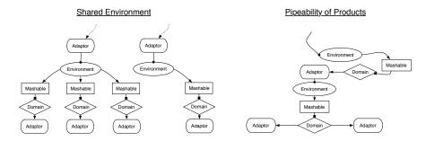
Fig. 5. Possible mashup graph configurations.
