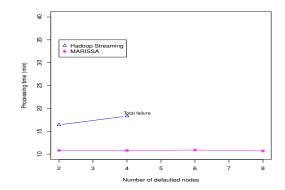
Fig. 9. This graph shows how Hadoop streaming and MARISSA behave faced with defaulting or dying nodes while running BLAST, processing 10240 genetic sequences. Both clusters start with 20 nodes, and progressively, in separate runs lose 2, 4, and 6 nodes. The Hadoop streaming framework however experiences a total failure beyond a 4 node loss. This occurs as worker nodes also hold vital data for processing.
