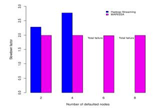
Fig. 10. This graph shows how Hadoop streaming and MARISSA slowdown given node losses while running BLAST. Both frameworks start with 20 nodes and process 10240 genetic sequences. Where comparable, Hadoop performs up to three times as slow, while MARISSA only slows down by a factor of 2.
