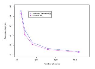
Fig. 8. MARISSA and Hadoop streaming cluster running BLAST, performing similarity comparisons on 40,960 genetic sequences. The number of cores used here varies from 10 to 160 cores.
