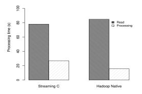
Fig. 3. Following **Table I** and **Figure** 2, this shows streaming performance as not a factor of I/O speeds in this case. In fact 'C" streaming performs faster I/O than Hadoop native. The performance losses occur in processing. This graph shows processing of 1.6TB of Wikipedia data being filtered to isolate embedded indices using 75 nodes in both cases.
