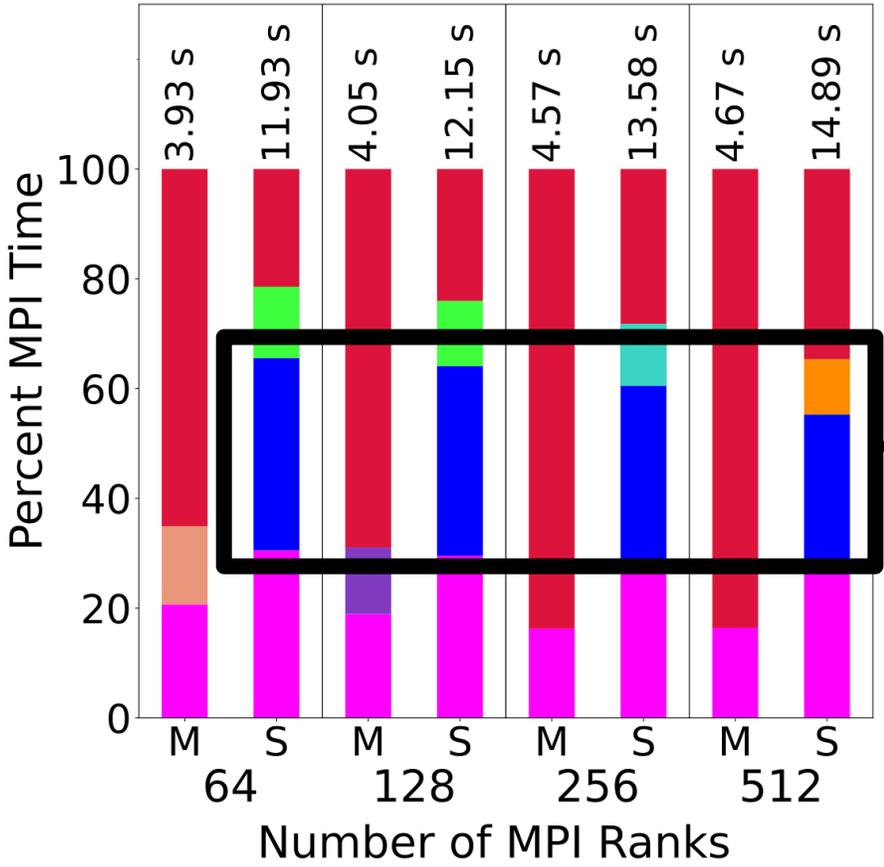
Spectrum-MPI uses libmlx5 (Mellanox InfiniBand driver) much more than MVAPICH
