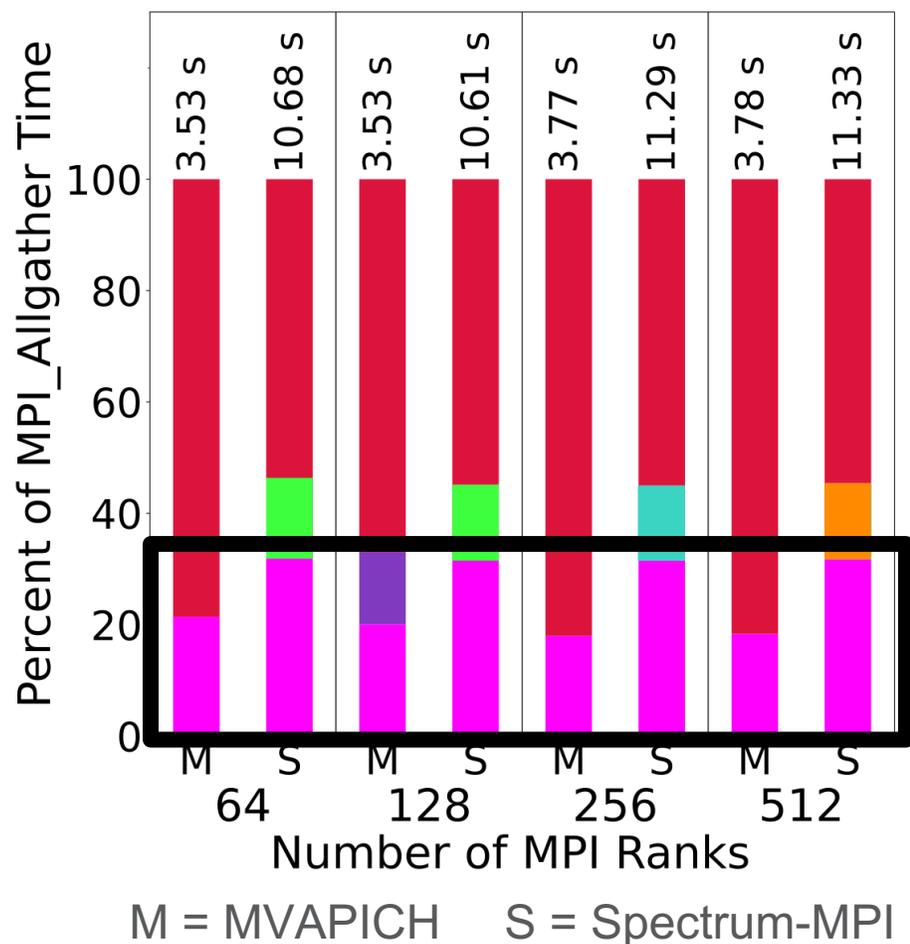
Spectrum-MPI uses pthread\_spin\_lock for a larger percentage of its time in MPI\_Allgather than MVAPICH
