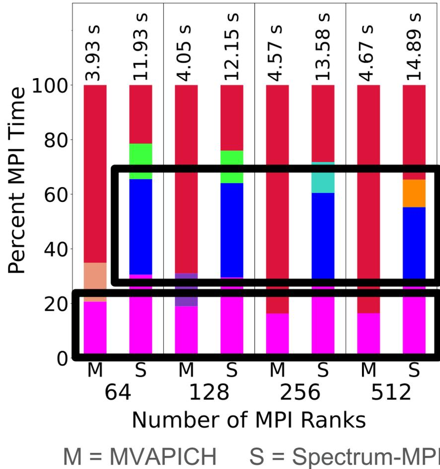
Spectrum-MPI uses libmlx5 (Mellanox InfiniBand driver) much more than MVAPICH
