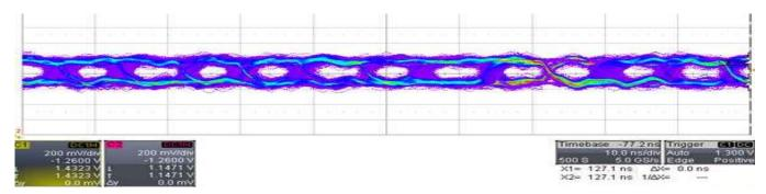
Fig. 5. Eye diagram of the SerDes link produced using the LeCroy High Frequency Oscilloscope
