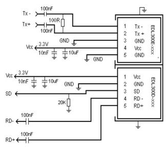
Fig. 4. LVDS SerDes Transmitter/ Receiver
