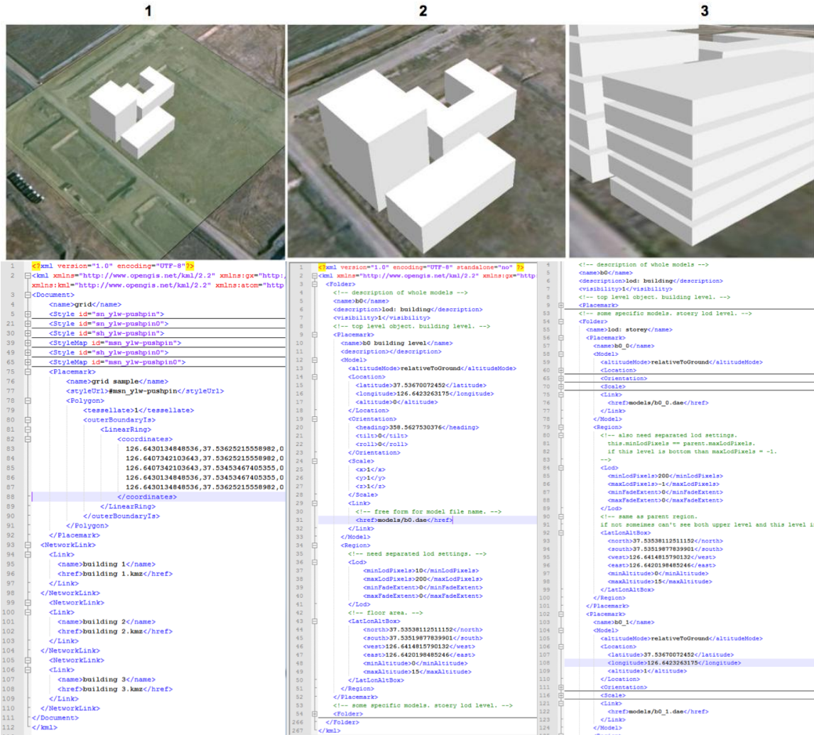
Figure 4 LOD scheme by KML 1. Building model in Grid cell, Grid cell has link to each building 2. Building unit: base area x number of floors, each Building has link to floors 3. Floor level of detail
