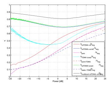
Fig. 3. Normalized throughput as a function of the average transmit power.
