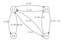
Fig. 1. Finite-state machine diagram for the cdTDMA+ALO protocol.
