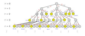
Fig. 2. Time evolution with time  $\tau$  of the cdTDMA+ALO protocol.
