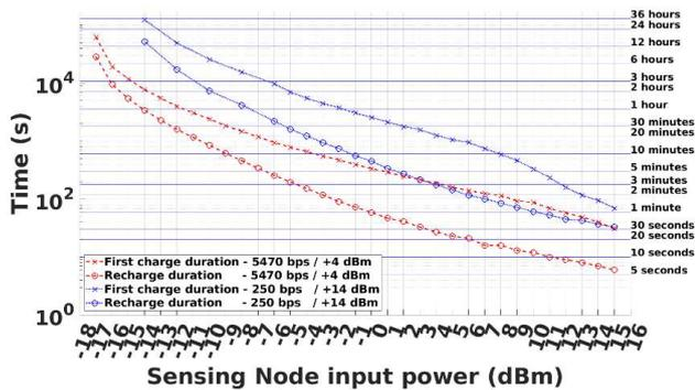
(b) Durations of the first charge ('x') and recharges ('o') against the conducted electromagnetic input power applied at the input of the rectifier of the Sensing Nodes, for a frequency of 868 MHz, and for two configurations of the wireless communication: transmission power of +4 dBm and data-rate of 5470 bps (dashed lines), and transmission power of +14 dBm and data-rate of 250 bps (dotted lines).
