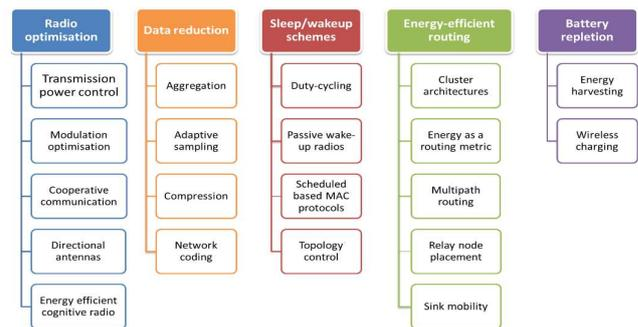
Fig. 3. Classification of WSN energy efficient mechanisms [14].
