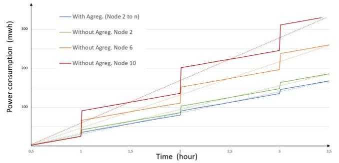
Fig. 9. Energy consumption profiles for intermediate nodes in a chain with a 1-hour collection period
