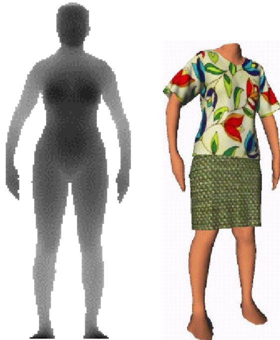
Figure II-8: Collision Detection using Z-buffer maps [VASS 01]
