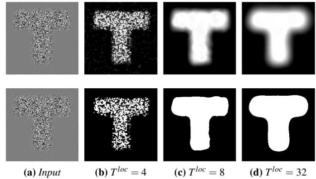
**Figure 7:** Computation of masks  $M_k$  from an SV-noise input (a). Top row: normalized distances  $\|S_x^{loc} - S_k^{loc}\|$ . Bottom row: binary masks. The larger  $T^{loc}$  the better the discrimination but the less precise the boundaries. A good strategy is to set  $T^{loc}$  as small as possible to get precise masks while still discriminating regions.
