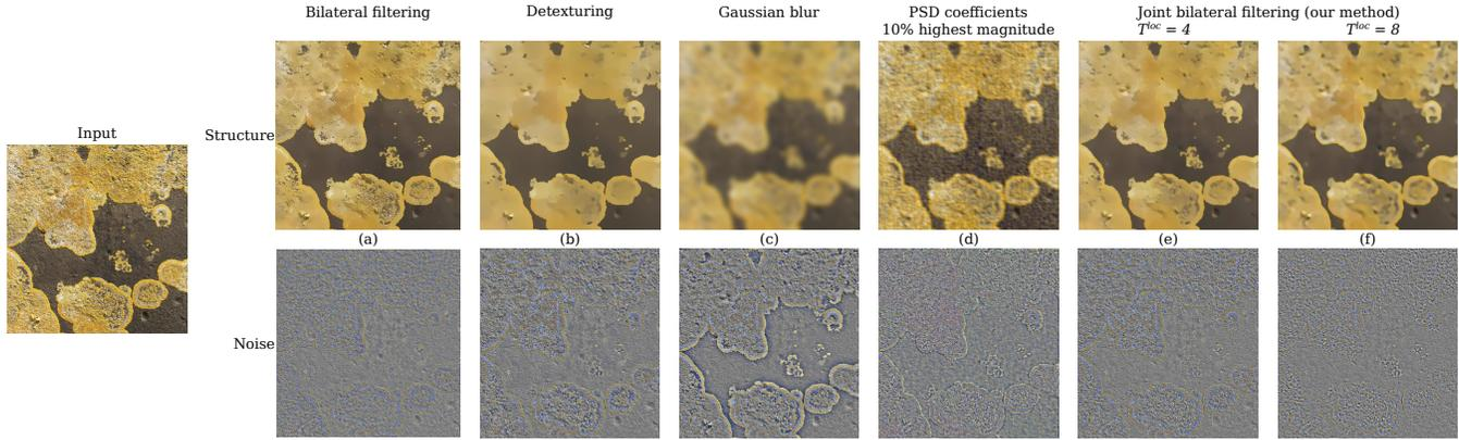
**Figure 13:** Structure extraction. Bilateral filtering and de-texturing perform well in some cases. Gaussian smoothing blurs sharp edges. Thresholding the PSD fails when high frequencies contribute to the structure. Our joint bilateral filtering driven by local spectra is versatile.
