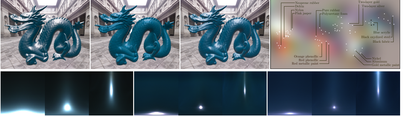
Figure 10: Real-time exploration of our BRDF manifold. 3 materials (circle points) are chosen manually, in the vicinity of blue-acrylic, by clicking in the 2D latent space (top right). The latent variables were optimised using all 100 materials of the MERL database. Our proposed construction of the BRDF manifold lends itself to real-time rendering (25 fps) using interpolated materials along with all combinations of dynamic geometry, view points and lighting (see sec. 5.1) using zonal harmonics up to L = 40 [SBN15]. The slices of the interpolated BRDFs are also visualised. Please see the accompanying video for a live demonstration.
