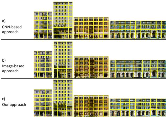
**Figure 13: Comparison of Façade Subdivision.** The top row shows the façade subdivision by a CNN-based method, which uniformly subdivides the façade based on the estimated floor height and column width. The second row shows the results by an image-based method using predefined numbers of floors and columns to estimate the floor height and column width. The bottom row shows improved subdivision by our approach.
