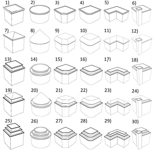
**Figure 3: Building Mass Grammars.** We define 30 grammars for the building mass in a systematic way. The first row defines single stack buildings with different footprints. The second row of buildings has the same footprints but have different roof shapes. The third and fourth rows show buildings with two stacks of masses, whereas the buildings in the bottom row have three stacks of building masses.
