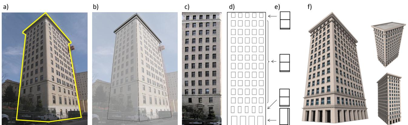
**Figure 1: Procedural Modeling from a Single Image.** a) Given an image and a silhouette of a building, b) our approach automatically estimates the camera parameters and generates a building mass grammar as a first step. Then, c) the façade image is rectified, and d) the façade grammar is generated. e) For each window non-terminal, the best window grammar is selected by maximum vote. f) Finally the output grammar is constructed and a corresponding 3D geometry is generated.
