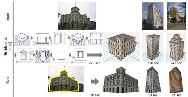
**Figure 9: Building Generation Comparison.** [NGDA\*16] requires the user to draw each element (i.e., building mass, roof, and windows), which takes around 4 minutes, and the fixed viewpoint makes it difficult for the user to sketch a target building. In contrast, our approach needs only a few user drawn lines and then computes a result fully automatically.
