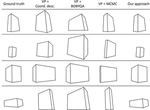
**Figure 10: Visual Comparison of Building Mass Generation.** Given a silhouette of the ground truth image, the estimation results are compared between our approach and other non-CNN based approaches. Estimation by other approaches is very poor even though the camera parameters are precisely estimated by the vanishing point approach.
