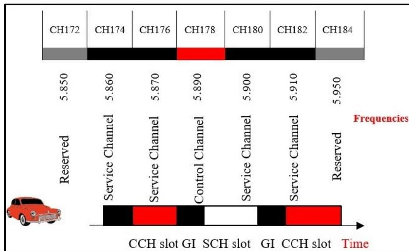
Figure 1 DSRC spectrum frequencies and IEEE1609.4 protocol operations
