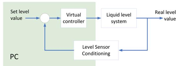
**Fig. 4.** Laboratory of liquid level control scheme
