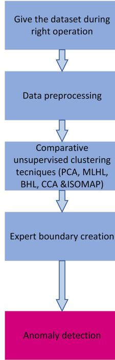
**Fig. 5.** Process Flowchart
