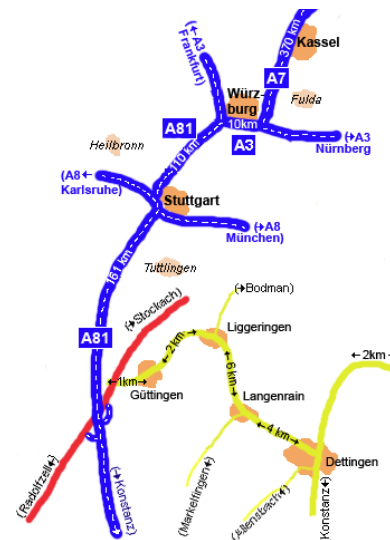
Figure 3: A hand-drawn sketch of a street network according to our design principles. It allows navigation from node to node by using town names on traffic signs, but also shows cities left and right of the path to support orientation.
