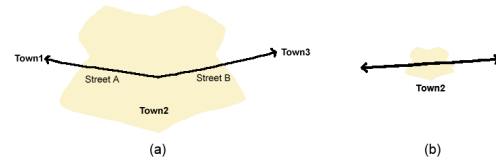
Figure 8: One example of an importance rating heuristic: If a village is passed, and the combined length of streets inside the village is less than 2 miles, the number of streets inside the village is 3 or less, and the maximum turning angle from street to street is less than 20 degrees, then the small village is passed almost straight through. The node (a) is tagged 'unimportant' and replaced by a simplified view (b).
