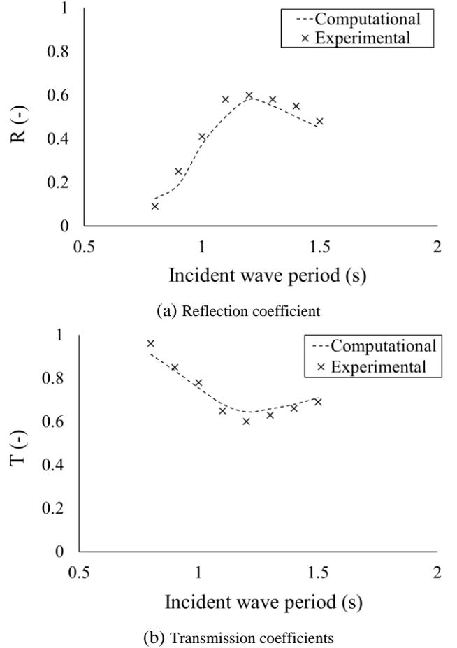
**FIGURE 7.** Comparison of reflection and transmission coefficients between computational and experimental (Liu, Huang, & Tan, 2009) data.
