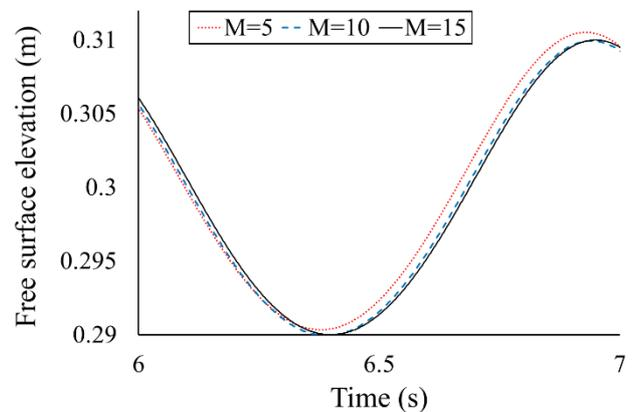
FIGURE 5. Downstream free surface elevation obtained using various cell numbers per wave height. The simulated wave condition is with  $T_w = 1.1$  s and  $H = 0.02$  m.
