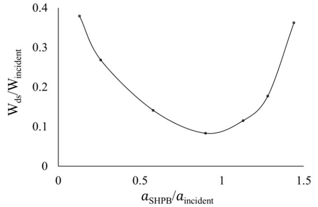
**FIGURE 17.** Downstream wave energy normalized by incident wave energy ( $W_{ds}/W_{incident}$ ) as a function of deformation amplitude of the SHPB normalized by the incident wave amplitude ( $a_{SHPB}/a_{incident}$ ), which changes due to varying  $AR$  of the SHPB. The applied wave condition in this figure is  $T_w = 1.1$  s and  $H = 0.02$  m.
