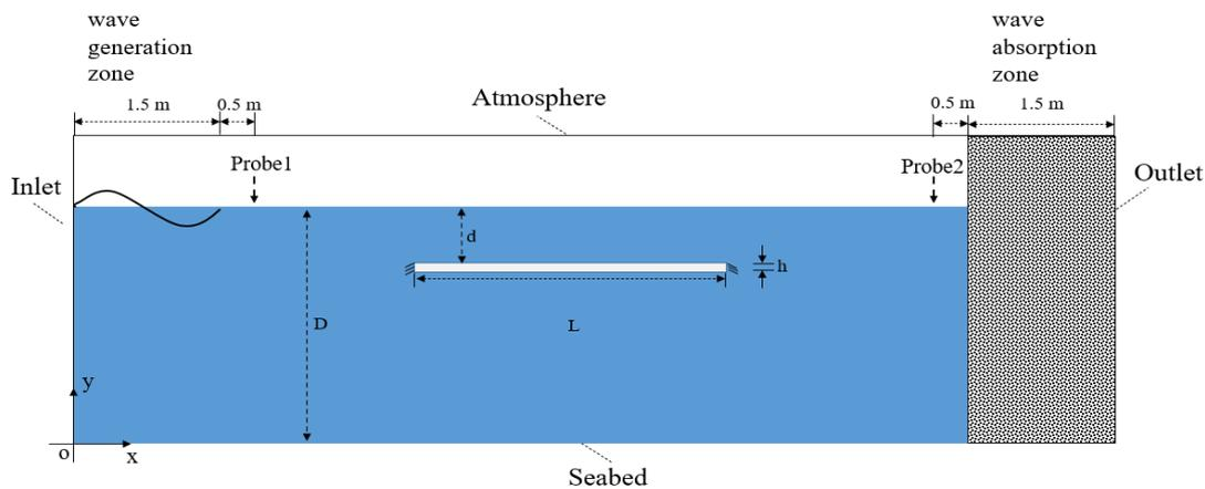
**FIGURE 2:** The computational model: in a numerical wave tank, a submerged horizontal plate is placed, whose upper and lower boundaries are deformable, while left and right boundaries are clamped. The domain is designed in a model scale to allow validation against experiments, whilst the scale factor is approximately 1:30 to real life.
