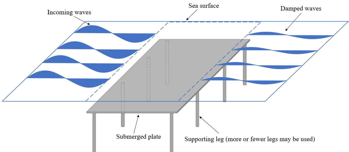
**FIGURE 1.** Sketch of a submerged-horizontal-plate breakwater; in real life, the device can be approximately 20 m long, 100 m wide and 0.4 m thick (Okubo, Takahashi, Kojima, & Moritaka, 1994; Wang, 2017; He, Gao, Xu, Ren, & Wang, 2019).
