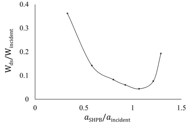
**FIGURE 15.** Downstream wave energy normalized by incident wave energy ( $W_{ds}/W_{incident}$ ) as a function of deformation amplitude of the SHPB normalized by the incident wave amplitude ( $a_{SHPB}/a_{incident}$ ), which changes due to varying  $E$  of the SHPB. The applied wave condition in this figure is  $T_w = 1.1$  s and  $H = 0.02$  m.
