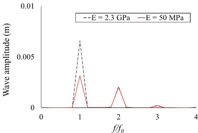
**FIGURE 10.** Comparison of downstream wave amplitude at different frequencies, between the flexible and stiff materials.  $f/f_0$  denotes the breakdown frequencies of downstream waves normalized by the incident wave frequency i.e.  $f_0 = 1/T_w$ . The applied wave condition in this figure is  $T_w = 1.1$  s and  $H = 0.02$  m.
