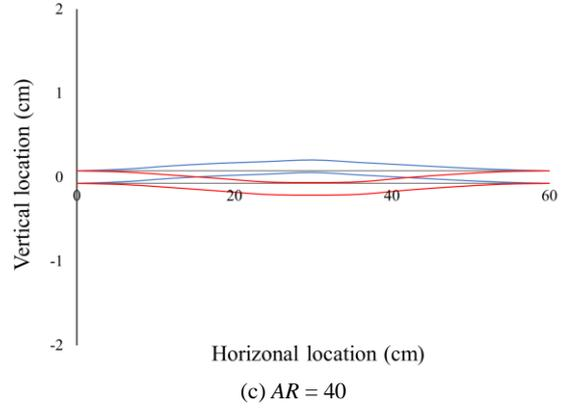
**FIGURE 16.** Upward and downward limits of the wave-induced SHPB deformation, obtained with plates of different aspect ratios. The applied wave condition in this figure is  $T_w = 1.1$  s and  $H = 0.02$  m.
