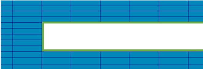
(b) Zoom-in fluid mesh around the left edge of the plate
