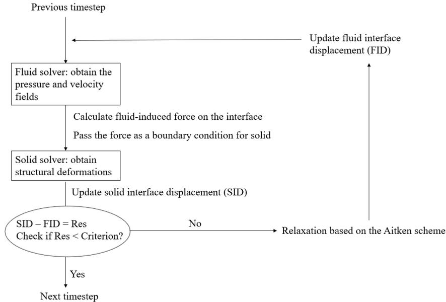
FIGURE 4. Solution procedure of the FSI inner loop.
