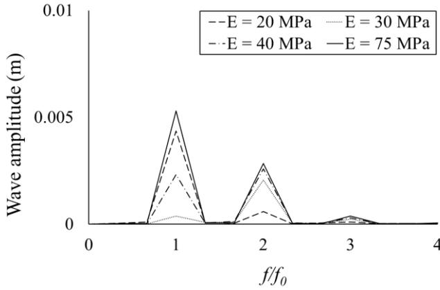
**FIGURE 14.** Comparison of downstream wave amplitudes at different frequencies, with a range of  $E$  applied to the SHPB. The applied wave condition in this figure is  $T_w = 1.1$  s and  $H = 0.02$  m.
