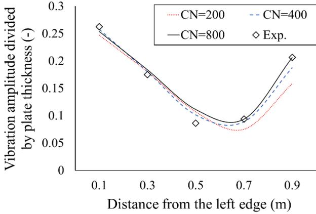
**FIGURE 6.** Plate deformation obtained with varying cell numbers (CN) for the solid mesh, comparing with the measurements of Sree, Law, & Shen (2017). The plate length is 1 m in total and the  $x$ -axis shows the measured distance from its left edge.
