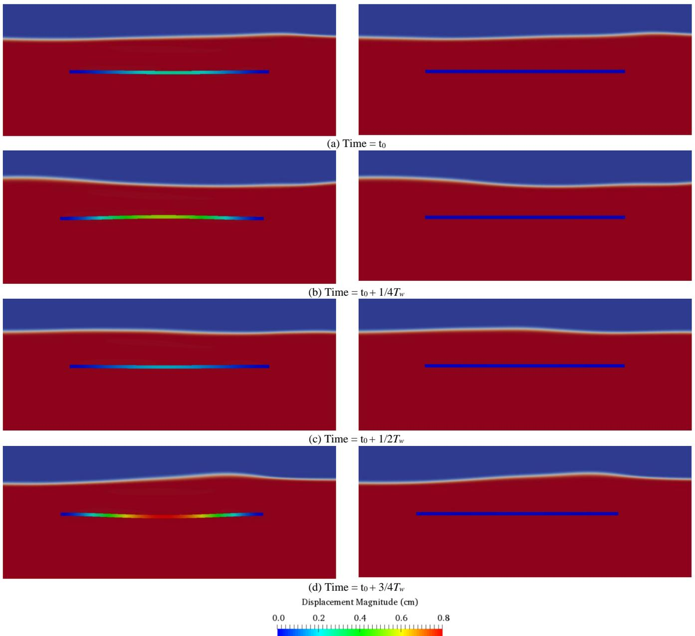
**FIGURE 8.** Comparison of wave-SHPB interaction between the flexible (left) and stiff (right) materials. The applied wave condition in this figure is  $T_w = 1.1$  s and  $H = 0.02$  m. In the subfigures, in red beneath the free surface is the water phase while in blue above the free surface is the air phase.
