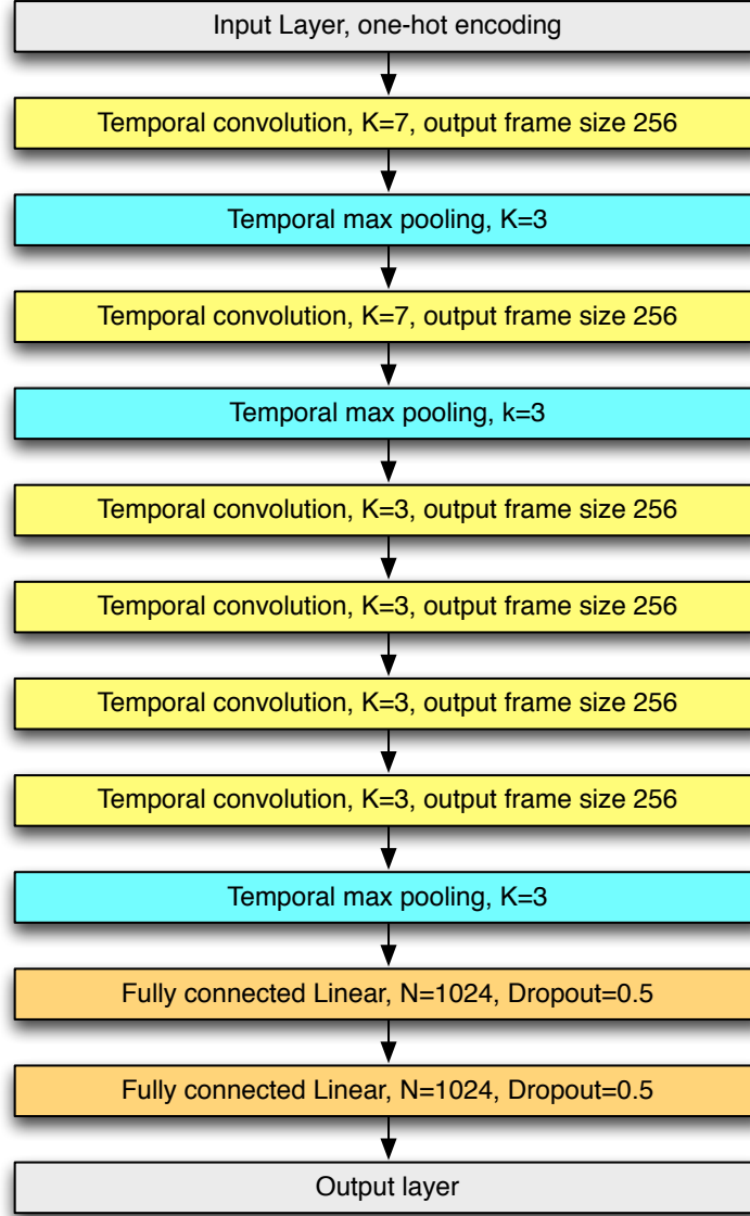
Figure 3: This is the basic network used in the experiments. The convolution layers are shown in yellow and correspond to the temporal convolution function described in Eq. 1. The max pooling layers are shown in blue and correspond to the function shown in Eq. 2. The fully connected layers at the bottom of the network are shown in orange. Included in the fully connected layer is a dropout of 0.5, which simply means half of the connections are dropped, and is used to prevent overfitting (Srivastava et al., 2014).
