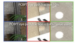
**Figure 15:** Increasing the number of eye-paths stored for caching does not have a large influence on results, in most regions of the image (insets same as Fig. 12). Computation times are respectively 5 min (below) and 28 min (above), for 167 iterations.
