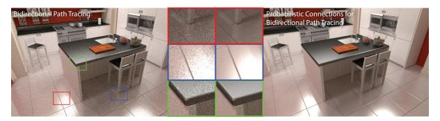
**Figure 1:** Our Probabilistic Connections for Bidirectional Path Tracing approach importance samples connections to an eye sub-path, and greatly reduces variance, by considering and reusing multiple light sub-paths at once. Our approach (right) achieves much higher quality than bidirectional path-tracing on the left for the same computation time (~8.4 min).
