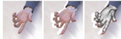
Fig. 1. The user's hand posture is estimated in real-time by fitting a 3D hand model to the Kinect point cloud using inverse kinematics.
