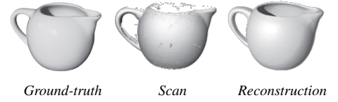
Figure 4: Reconstruction using the method of Pauly et al. [PMG*05]. This technique can cope with large missing parts in scans, such as the other side of the creamer (upper part of the scan).
