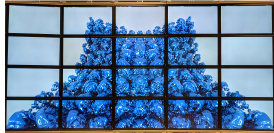
Figure 4: A prototype display wall system using DFB pixel operations to send tiles in parallel from an image-parallel path tracer.
