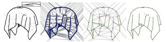
**Figure 3.1:** Algorithm Pipeline. From left to right: input point set; Delaunay triangulation of input; after simplification, with ghost edges in grey, relevant solid edges in green, discarded solid edges in red; final reconstruction.
