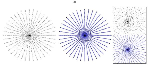
**Figure 4.5:** Noisy star. The lines of the inferred shape near the star center are visually indistinguishable (see closeup). Nevertheless, our method reliably recovers the lines and intersection point by interleaving decimation and relocation.
