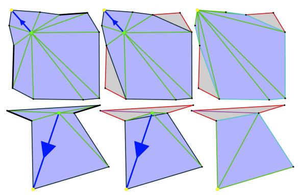
**Figure 3.5:** *Making edges collapsible.* Left: collapsing the edge (in blue) creates fold-overs because of blocking edges (in black). Middle: the flipping procedure makes the edge collapsible. Right: after collapse.
