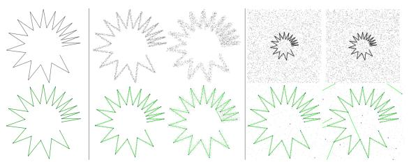
Figure 4.3: Robustness to noise and outliers. The input shape (3K points) has sharp corners subtending small angles as well as boundaries. Our reconstruction is perfect for a noise-free input (left); as noise is added (middle, 2% and 2.5% of bounding box), the output degrades gracefully, still capturing most of the sharp angles; even after adding 4K or 4.5K outliers and 2% of noise (right), the reconstruction remains of high quality, although artifacts start appearing in this regime.
