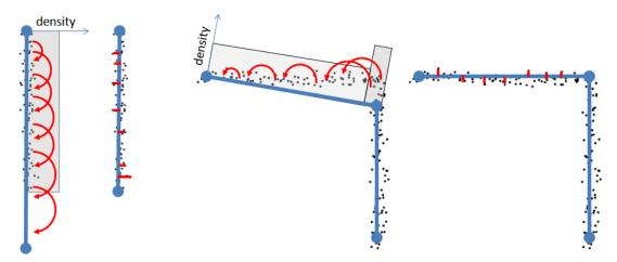
**Figure 2.1:** Boundary and feature preservation. Left: An edge extending beyond (or falling short of) the point set would incur a large tangential component, enforcing preservation of boundaries. Right: When an edge does not fit a sharp corner, the transport cost has both a large tangential component (due to the non-uniform sampling along the edge) and a large normal error. Minimizing transport cost will thus induce alignment of edges to features.
