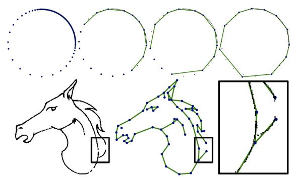
**Figure 5.1:** Sampling Density. Top: the transport cost favors the decimation of areas with high point density. As we further simplify the triangulation, regions with lower densities are also recovered. Bottom: areas with missing data are reconstructed as boundaries.
