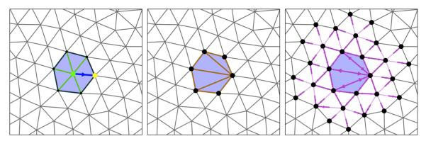
**Figure 3.4:** Updates during collapse. Left: collapse operator. Middle: edges with updated cost. Right: collapse operators pushed to the priority queue.
