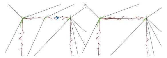
**Figure 3.3:** *Edge simplification. Half-edge collapse (arrow) triggers a local reassignment of the input points (assignments in red for edges, green for vertices).*
