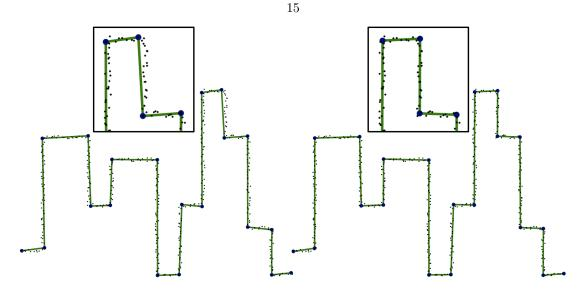
Figure 3.6: Vertex relocation. Noisy skyline point set, before (left) and after (right) vertex relocation.
