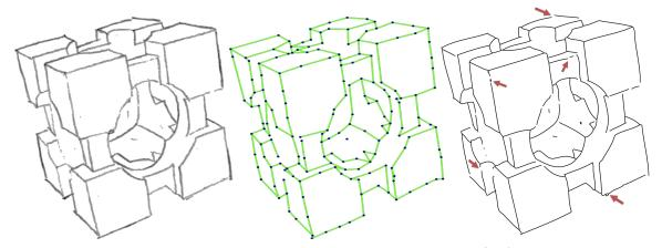
**Figure 4.7:** Mechanical part. Line drawing with complex features (left). Our reconstruction (middle) preserves intersection, corners, and manages to even remove small wiggles and glitches. In comparison, Adobe's Live Trace<sup>®</sup> fails to handle glitches of this sketch (red arrows).
