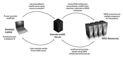
Figure 1 The three tier client/server architecture employed by multiR
