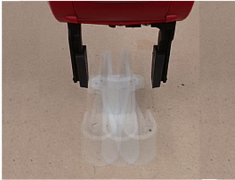
FIGURE 2. Illustration of perception uncertainty in the part location - Estimated posture might differ from the actual part posture.
