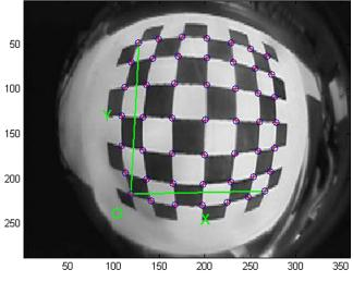
Fig. 7 Image points and reprojected grid points.
