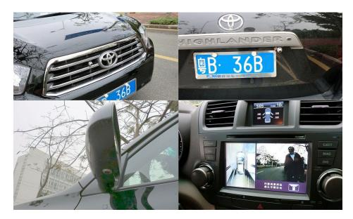
Fig. 5 PPAS installed in a Toyota Highlander.
