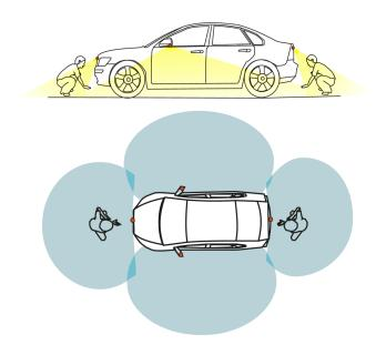
Fig. 1 Side view and top view of panorama parking assistant system (PPAS).
