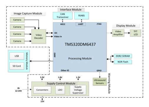
Fig. 4 System architecture for PPAS.
