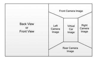
Fig. 2 Screen arrangement of PPAS.
