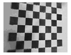
Fig. 9 The result of correction of the fisheye camera distortion after basic calibration.
