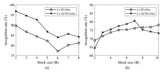
Fig. 5 Recognition rate of L1-PCANet and L1-2D<sup>2</sup>PCANet on extended Yale B and FERET dataset for varying number of block size. (a) Extended Yale B and (b) FERET.
