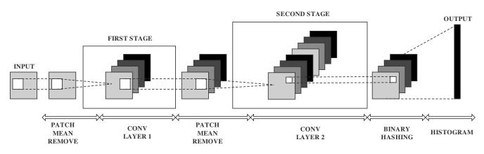
Fig. 2 The illustration of two-layer L1-2D<sup>2</sup>PCANet.
