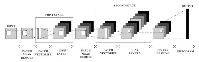
Fig. 1 The illustration of two-layer L1-PCANet.
