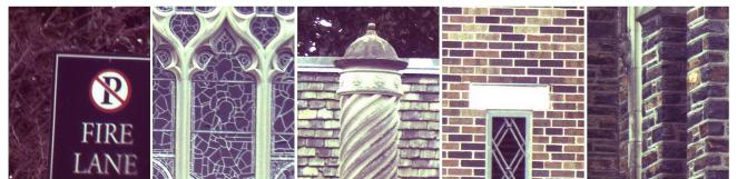
Figure 3: Zoomed in regions of Fig. 2 showing the detail of the AWARE 10 camera system. Distance to object from camera, Left to right: 54m, 162m, 123m, 117m, 162m.
