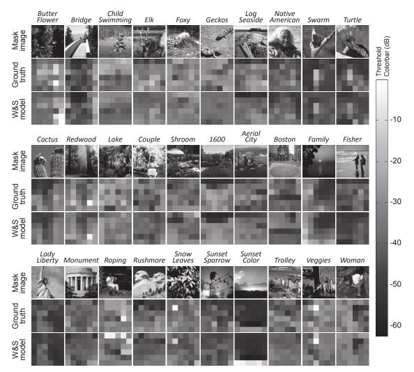
Figure 2. Local masked detection thresholds and model predicted thresholds for images from the CSIQ image-quality database (see text for details).
