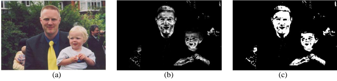
Figure 6: (a) Our original image, (b) its corresponding skin likelihood image, and (c) the segmentation achieved through the application of a 0.5 probability threshold.
