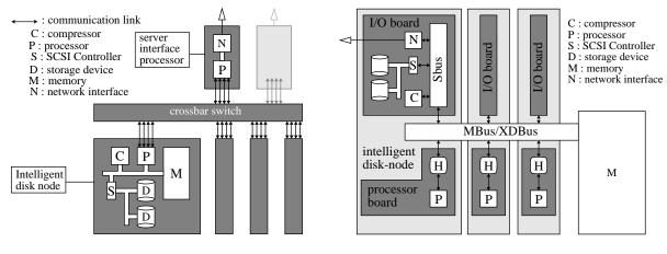
Figure 2 : Point to point architecture
