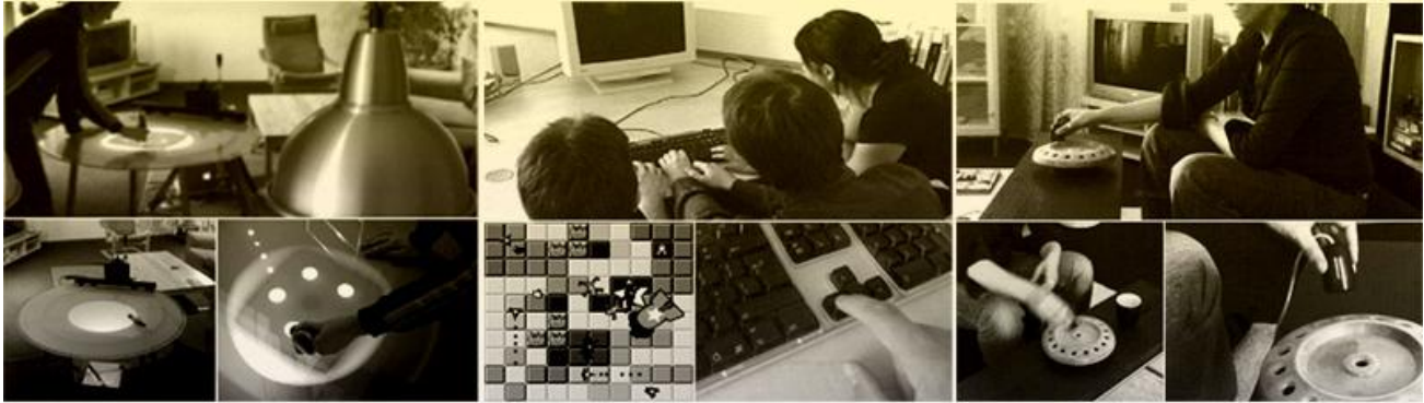
Fig. 1: Impression of the three prototypes. From left to right: digital pool table, multi-player video game called “Game of Flight” and voicemail browser. In the game of pool a pen is used to manipulate the movements of virtual balls projected from underneath. The video game is presented in an audiovisual format on a desktop computer and contains an aircraft-avatar that can be manipulated via keys on the keyboard. The voicemail browser comprises 16 voicemail slots along its ridge with one voicemail message per slot. The messages can be accessed by performing gestures above the slots. The middle slot serves as a base for the input device. Pictures taken from Rozendaal 21 .
