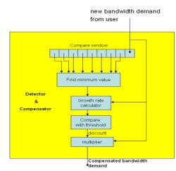
Fig. 3. Block diagram of strategic node detector and compensator.
