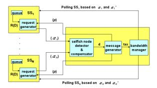
Fig. 2. Block diagram of SBPM in a WiMAX network.
