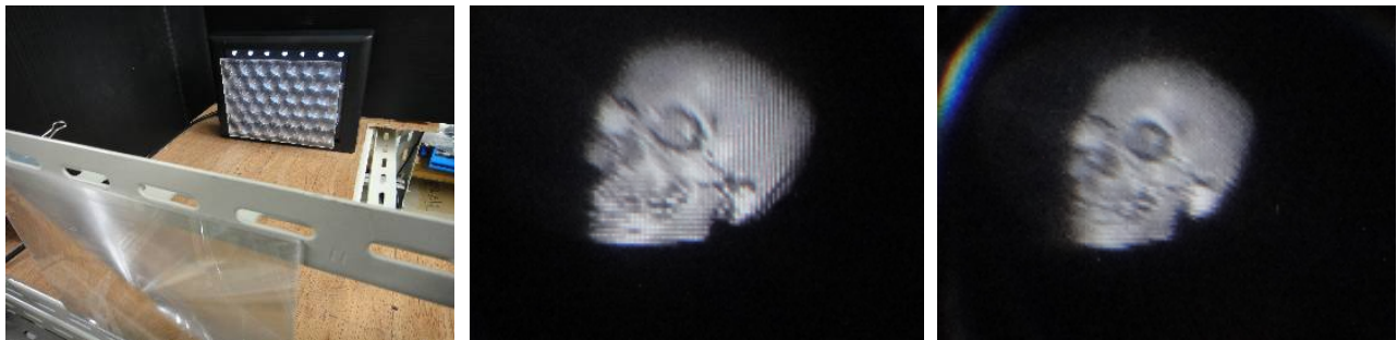
Figure 4. Prototype system A (left) and the images observed from central viewpoint (middle) and a far-left viewpoint (right) with this system.
