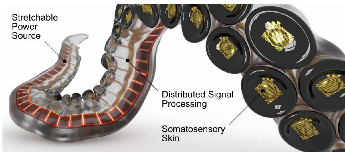
Fig. 1. Narrowing the gap between biological and robotic systems. All-soft robots ideally integrate soft actuation with stretchable, multimodal electronic skins and energy supply. Untethered autonomous operation is the ultimate goal.
