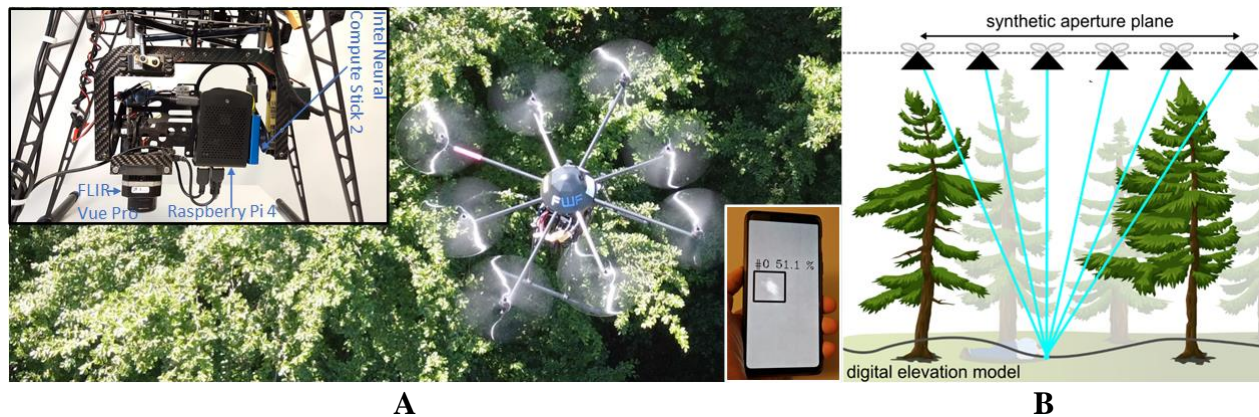
Figure 1. Autonomous drone supporting search and rescue missions. (A) Camera drone with the recording and processing equipment used in our experiments. In the case of a positive finding, an integral image with classification result and location is transmitted to a mobile device of the rescue team. (B) Basic principle of airborne optical sectioning (AOS). Supplementary Movie S1 shows video footage of drone and sample test site.
