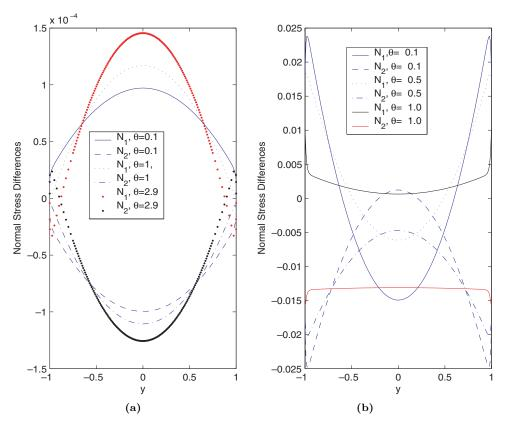
FIG. 5. The normal stress differences  $N_1$  and  $N_2$  in tumbling regimes as functions of y at selected values of  $\theta$  with tangentially anchored boundary conditions in weak shear. (a) Rods:  $a=0.8, N=6, De=0.01, Er=100, \alpha=10, \mu_1=0.01, \eta=0.02$ . (b) Discs:  $a=-0.8, N=6, De=0.01, Er=100, \alpha=10, \mu_1=-0.01, \eta=0.02$ .
