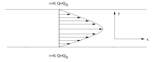
Fig. 10. The geometry of the plane Poiseuille flow. A pressure gradient  $\frac{\partial p}{\partial x} = -De^2$  is imposed across the channel. At the bounding surfaces, the orientation tensor is assumed to equal to its equilibrium value.
