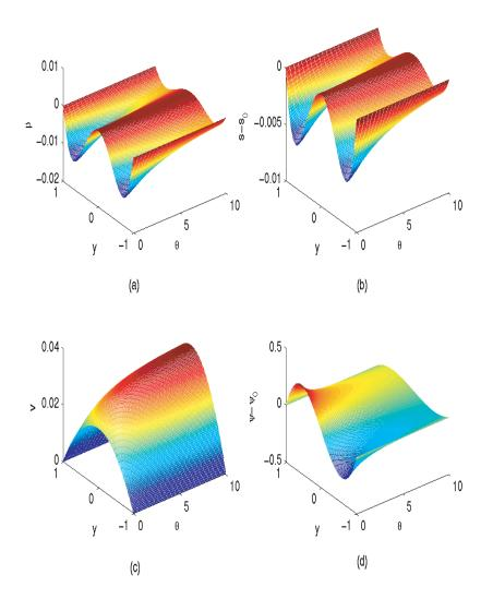
FIG. 14. Steady solutions  $\beta, s-s_0, v$  and  $\psi-\psi_0$  for tumbling rods as functions of  $(\theta, y)$  with normally anchored boundary conditions in plane Poiseuille flows. The parameter values are  $a=0.8, N=6, De=0.01, Er=100, \mu_1=0.01, \eta=0.02, \alpha=1$ .
