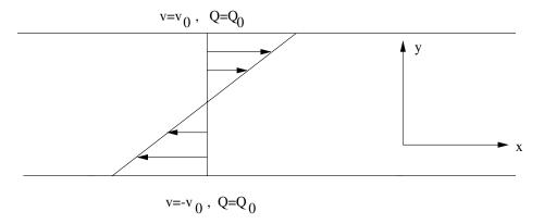
Fig. 1. Geometry of plane Couette flow. The gap width in the shear cell is 2h. The LCP in the cell is sheared by moving the upper plate with a constant speed  $v_0$  and the lower one with the same speed in the opposite direction. At the bounding surfaces, the orientation tensor is equal to its equilibrium value.
