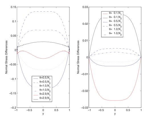
FIG. 12. The normal stress differences  $N_1$  and  $N_2$  as functions of y in tumbling regime at selected values of  $\theta$  with tangentially anchored boundary conditions in plane Poiseuille flows. The other parameter values are N=6, De=0.01, Er=100,  $\alpha=10$ ,  $\mu_2=0.02$ , for rods a=0.8,  $\mu_1=0.01$ , and for discs, a=-0.8,  $\mu_1=-0.01$ .
