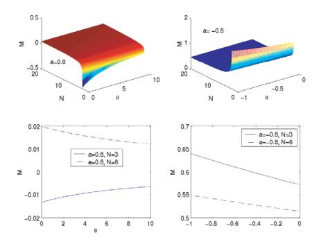
Fig. 2. M as a function of N and  $\theta$  with tangentially anchored boundary conditions in weak Couette flow: The top left panel is for rods, with a=0.8, whereas the top right panel is for platelets, with a=-0.8. The bottom panels show M for two distinct concentrations of rods (left) and platelets (right).
