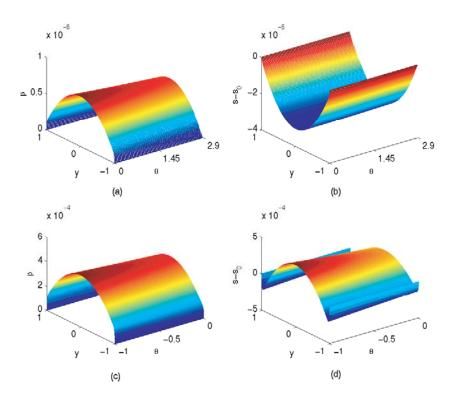
Fig. 4. The steady-state asymptotic solutions  $\beta$  (left column) and  $s-s_0$  (right column) in the tumbling regime as functions of  $(\theta,y)$  with tangentially anchored boundary conditions in weak Couette flows. (a) and (b) depict the solution for rods with parameter values a=0.8, N=6, De=0.01, Er=100. (c) and (d) depict the solution for discs with parameter values a=-0.8, N=6, De=0.01, Er=100.
