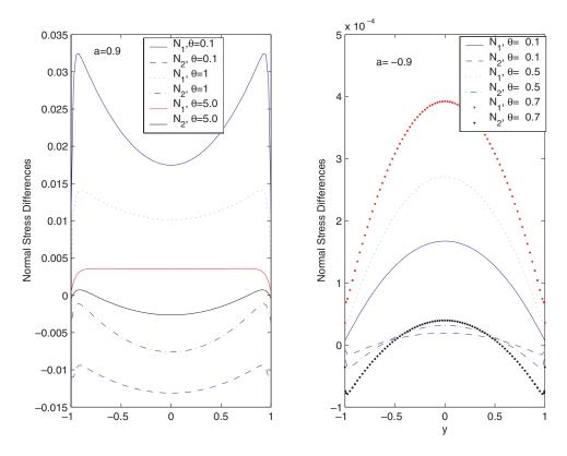
Fig. 9. The normal stress differences  $N_1$  and  $N_2$  as functions of y in flowing-aligning regime at selected values of  $\theta$  with normally anchored boundary conditions in weak shear. The parameter values are  $a=\pm 0.9, N=6, De=0.01, Er=100, \alpha=10, \mu_1=\pm 0.01, \mu_2=0.02$  for rods and discs, respectively.
