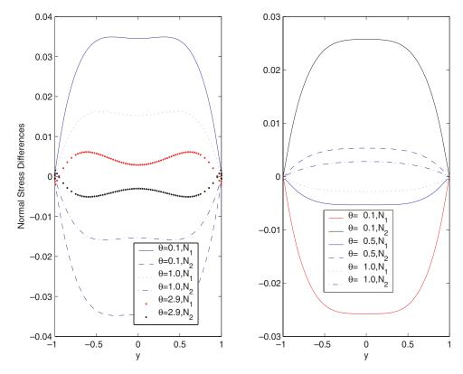
Fig. 13. The normal stress differences  $N_1$  and  $N_2$  as functions of y in flow-aligning regime at some values of  $\theta$  with tangentially anchored boundary conditions in plane Poiseuille flows. The other parameter values are N=6, De=0.01, Er=100,  $\alpha=10$ ,  $\mu_2=0.02$ , for rods a=0.9,  $\mu_1=0.01$ , and for discs, a=-0.9,  $\mu_1=-0.01$ .
