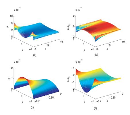
FIG. 7. The steady-state asymptotic solution as functions of  $(\theta, y)$  in tumbling regime with normally anchored boundary condition in weak shear. (a) and (b) depict the solution for rods with parameter values a=0.8, N=6, De=0.01, Er=100. (c) and (d) depict the solution for discs with parameter values a=-0.8, N=6, De=0.01, Er=100.
