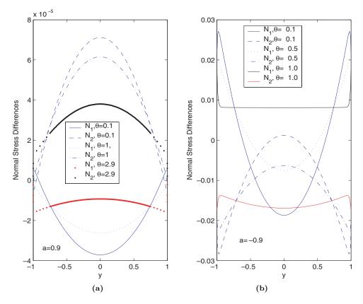
FIG. 6. The normal stress differences  $N_1$  and  $N_2$  in flowing-aligning regimes as functions of y at selected values of  $\theta$  with tangentially anchored boundary conditions in weak shear. (a) Rods:  $a=0.9, N=6, De=0.01, Er=100, \alpha=10, \mu_1=0.01, \eta=0.02$ . (b) Discs:  $a=-0.9, N=6, De=0.01, Er=100, \alpha=10, \mu_1=-0.01, \eta=0.02$ .
