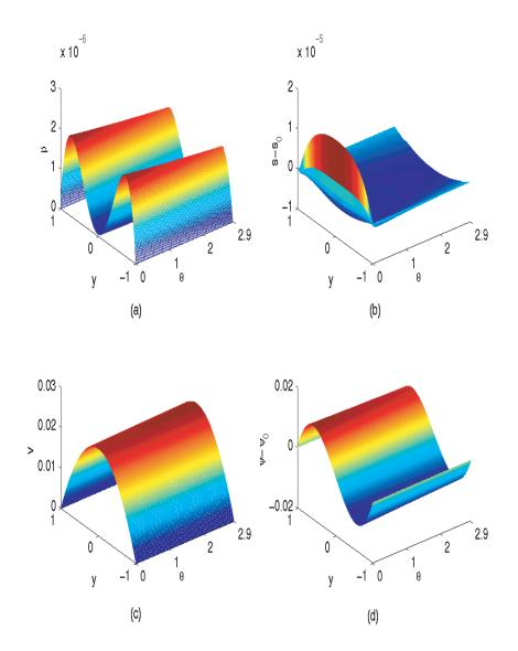
Fig. 11. Steady solutions of  $\beta$ ,  $s-s_0$ , v and  $\psi-\psi_0$  as functions of  $(\theta,y)$  in the regime of tumbling rods with tangentially anchored boundary conditions in plane Poiseuille flow. The parameter values are  $N=6, a=0.8, De=0.01, Er=100, \mu_1=0.1, \eta=0.2, \alpha=10$ .
