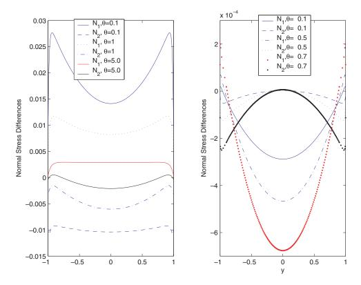
FIG. 8. The normal stress differences  $N_1$  and  $N_2$  as functions of y in tumbling regime at selected values of  $\theta$  with normally anchored boundary conditions in weak shear. The parameter values are  $a=\pm 0.8, N=6, De=0.01, Er=100, \alpha=10, \mu_1=\pm 0.01, \mu_2=0.02$  for rods and discs, respectively.
