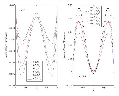
FIG. 15. The normal stress differences  $N_1$  and  $N_2$  as functions of y in tumbling regime at selected values of  $\theta$  with normal anchoring boundary conditions in plane Poiseuille flows. The parameter values are N=6, De=0.01, Er=100,  $\alpha=10$ ,, a=0.8,  $\mu_1=0.01$ ,  $\mu_2=0.02$  for rods, and a=-0.8,  $\mu_1=-0.01$ ,  $\mu_2=0.02$  for discs.
