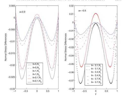
FIG. 16. The normal stress differences  $N_1$  and  $N_2$  as functions of y in flow-aligning regime at selected values of  $\theta$  with normal anchoring boundary conditions in plane Poiseuille flows. The parameter values are N=6, De=0.01, Er=100,  $\alpha=10$ , a=0.9,  $\mu_1=0.01$ ,  $\mu_2=0.02$  for rods, and N=6, De=0.01, Er=100, Er=10
